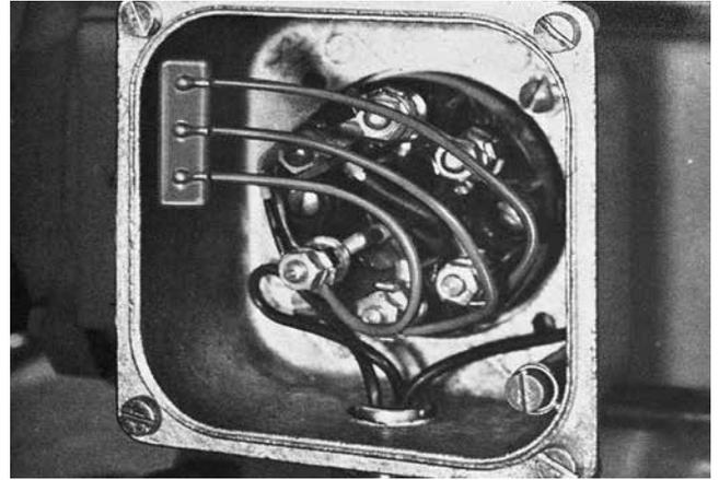
**THREE PHASE STAR-CONNECTED SURGE SUPPRESSOR CONNECTED INTO A MOTOR TERMINAL CONNECTING BOX.**
