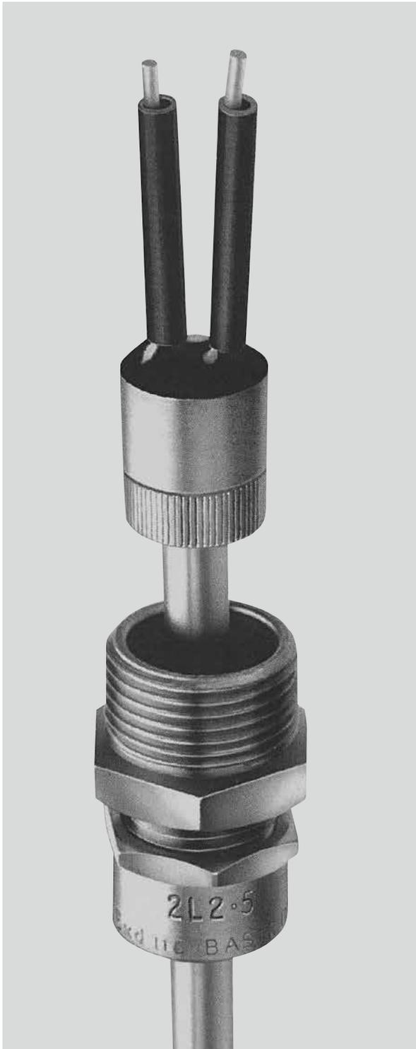
The insulator consists basically of a brass screw-on pot with a glass filling medium and is suitable for use at temperatures between 150°C and 250°C.
