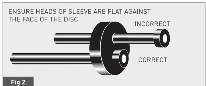
Slide the disc assembly over the conductors, and into the pot recess to check for fit, then partially withdraw. In the case of seven conductor cables, this operation can be facilitated by shortening the outer ring of conductors by 10mm. When terminating mutli-core cables with 10mm<sup>2</sup>, 16mm<sup>2</sup>, or 25mm<sup>2</sup> conductors, the conductors should be "set" within the pot to facilitate location of the disc assembly within the recess.
